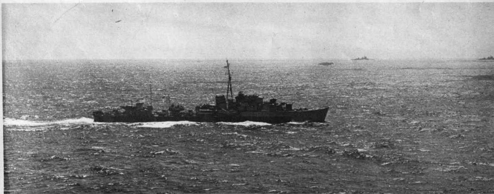
BRITISH DESTROYERS are low and stubby in profile. Superfiring turret and flash guard on "O" Class ship create a slope up to squat
